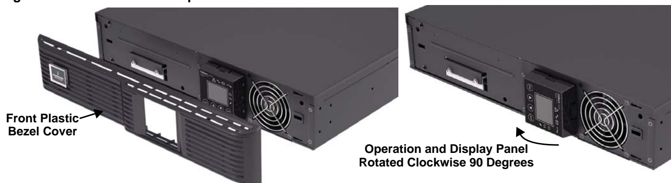
Figure 8 Remove the front plastic bezel cover
