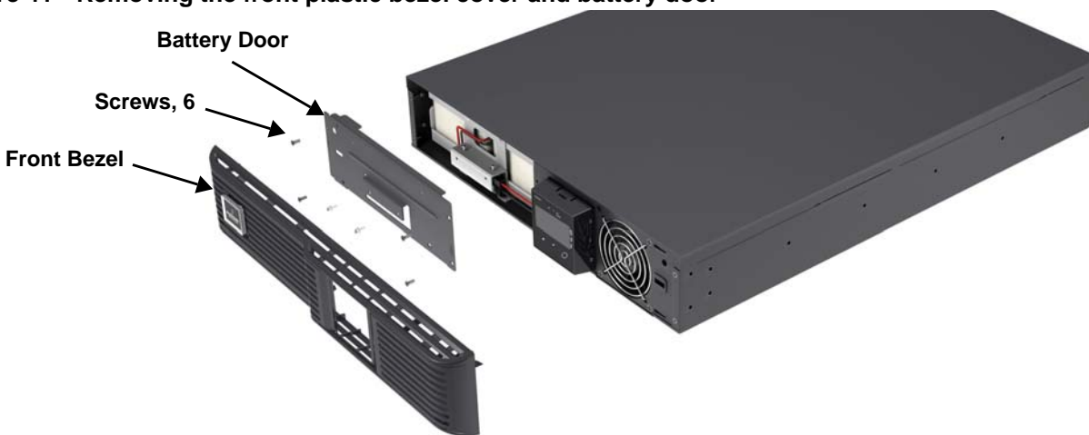
Figure 41 Removing the front plastic bezel cover and battery door
